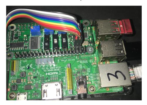
3. Until you are more familiar with the ICS-CTRL board, you might want to **take a fine tipped** marker and mark the IN, OUT and GAIN potentiometers. The GAIN potentiometer controls the amplification of the output amplifier (going to the transmitter microhone input) and works in conjunction with the (linear) OUT potentiometer, which is in a normal volume control configuration. This gives TREMENDOUS potential output variability in signal level!
