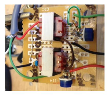
Note the resistors and the jumpers needed to make the required center tap and ground connections.
