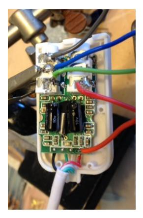
In this photo, the orange wire going near the big white USB cable, is picking off +V from the tiny soldering connection available there. This is a difficult soldering job, be careful. As an alternative, you can use a second USB cable, just to get to the red and black wires (+v and ground, respectively). This is a lot easier to accomplish mechanically!
