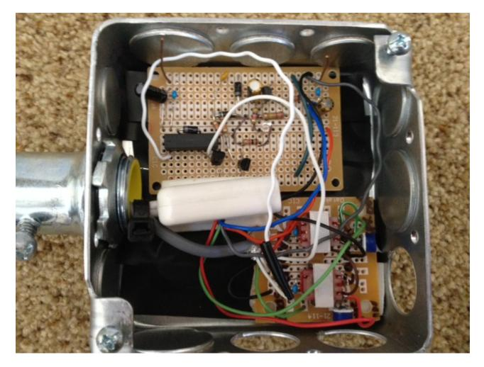
This is the entire circuitry inside an electrical box. One of our members has access to Tea tins, which are about 1 cup volume, and make mounting even easier, because you can double-stick tape to all of the inside walls. A 7/8" wood boring bit is used to cut a hole in the bottom of the tea-tin, and then the electrical sleeve is used to bush the sharp edge --- this could also be done with an appropriate rubber bushing.
