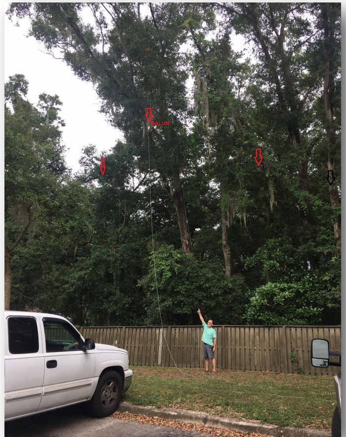
Figure 1: Photo of temporarily installed antenna, with center Balun at approximately 26 feet above ground. Inverted V type clone of a buckmaster antenna. Except for the light-colored RG8X coaxial cable, the antenna is almost invisible.
