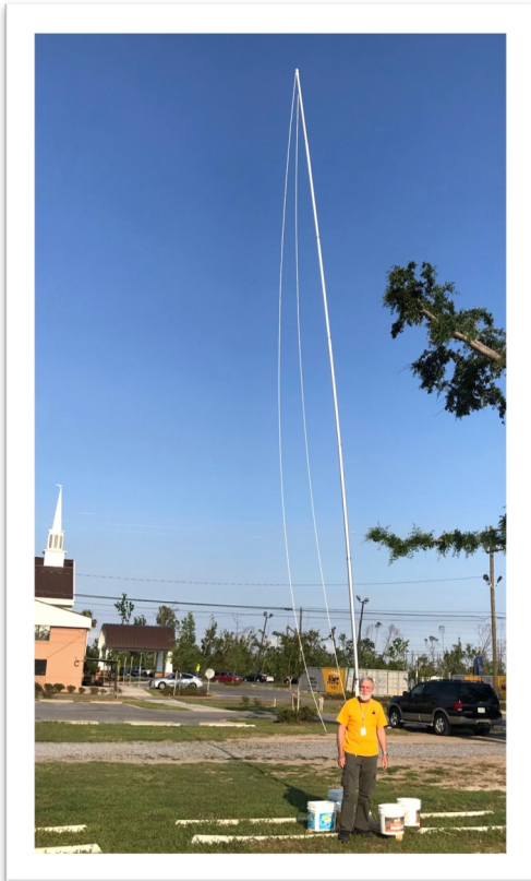
Tim Linn KD5SSF and his water-bucket stabilized telescopic ham radio antenna mast.
