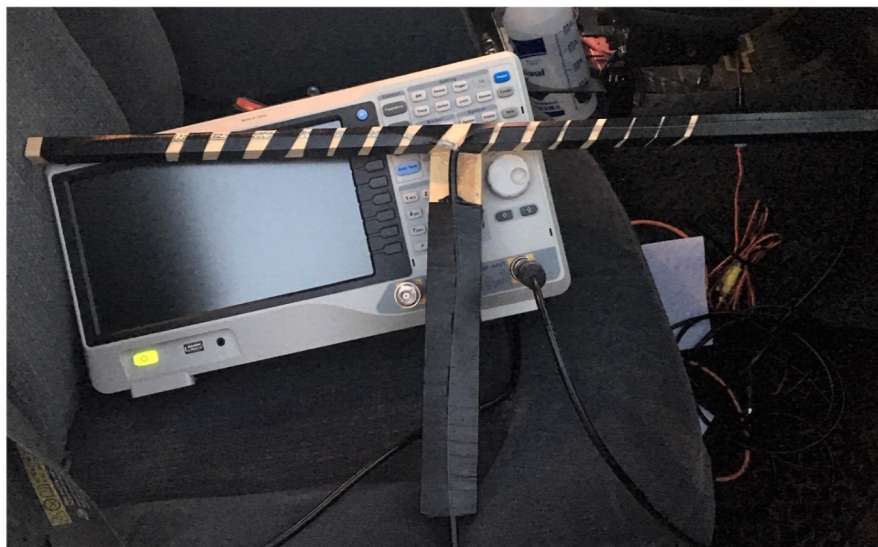
Figure 1. Homebrew small dipole to measure E-fields.
