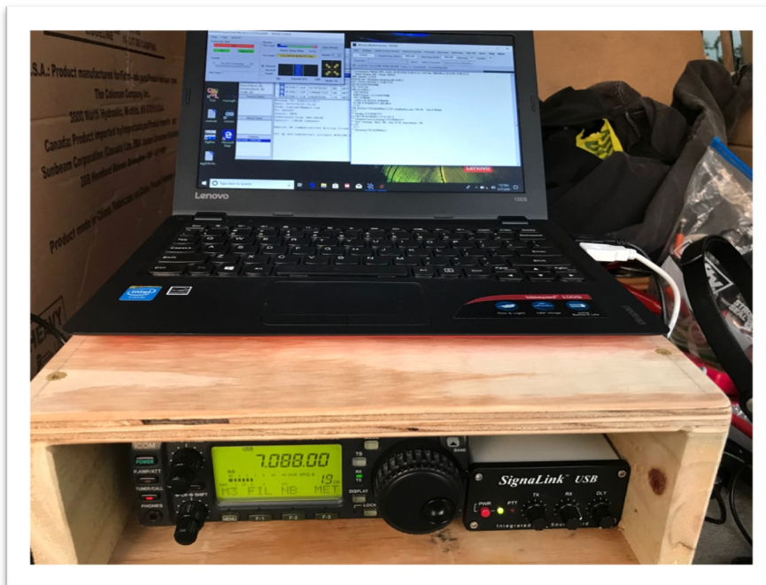
Tim has his WINLINK client connected to AJ4GU near Atlanta Ga, passing traffic on 40 meters. His go-box is assembled in a simple plywood box created by Stewart Reissener KK4DXF of the Alachua County ARES/NFARC group.
