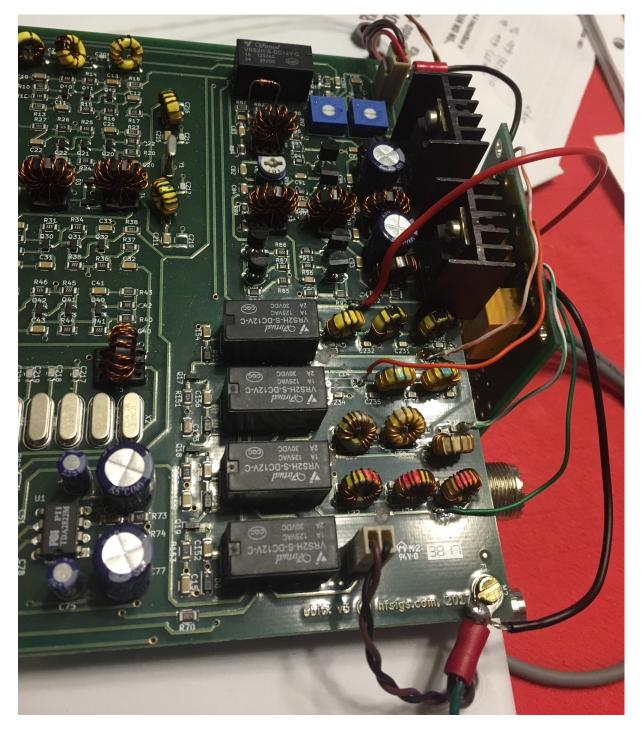
Be certain to ground the Daughter board in at least two locations on the uBitx board. You can see the black wires here going to the corner ground connections using ring terminals.
