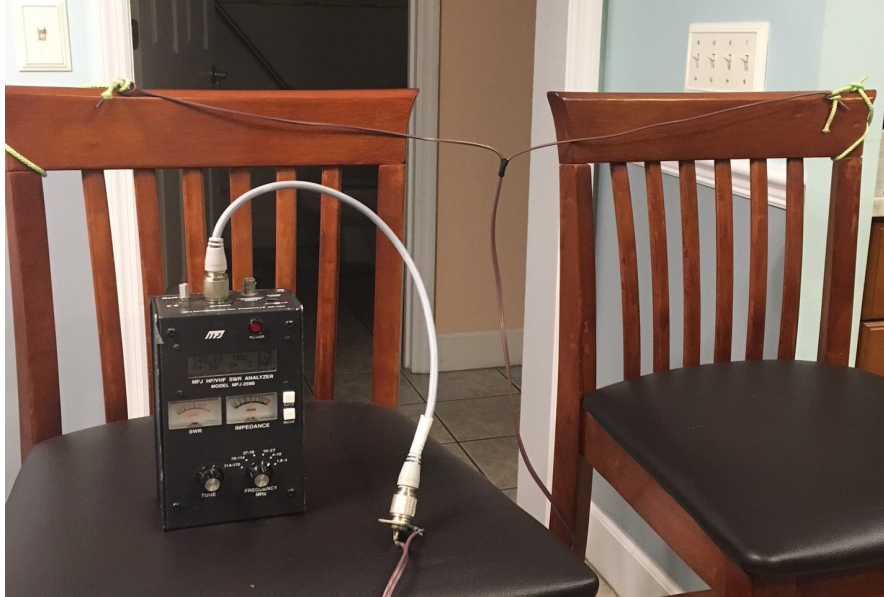
Figure. Very simple VHF antenna made from 2-conductor lampwire (#18, Home Depot). Rope as insulators on both sides, lampwire as transmission line. 34" dipole showed lowest SWR 1.2 around 143 MHz. Adjust as desired, tape center to set dimension.
