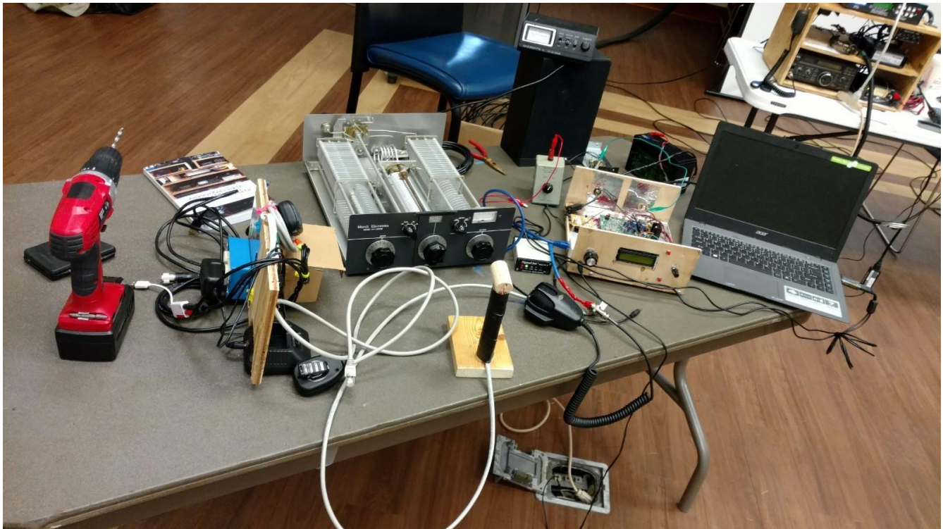
One of three tables full of gear for a distinctly hands-on Technician course. BitX40 transceiver in a plywood open housing just to the left of the laptop computer. It fascinated the students. We opened the antenna tuner so components and adjustments were more obvious. Homemade desk mic constructed using 1" dowel rod.
