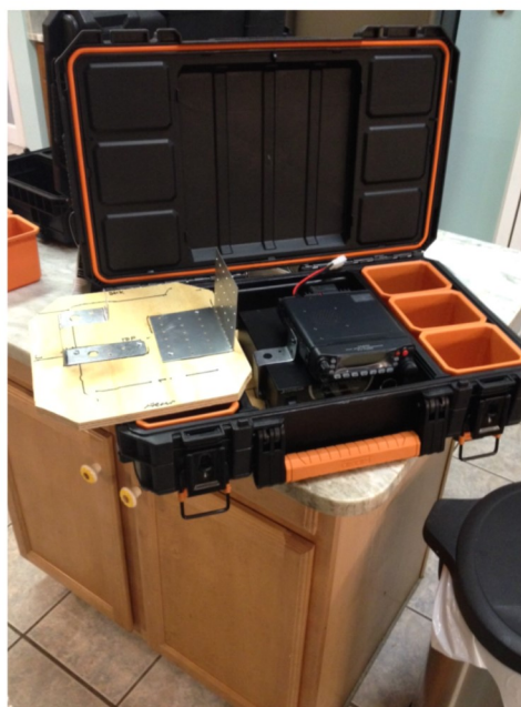
Mounting system to create waterproofed vhf transceiver go-box
