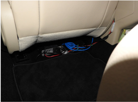
The main body of the Icom 880H affixed to the floor mat with Industrial Strength Velcro under the driver's seat.
