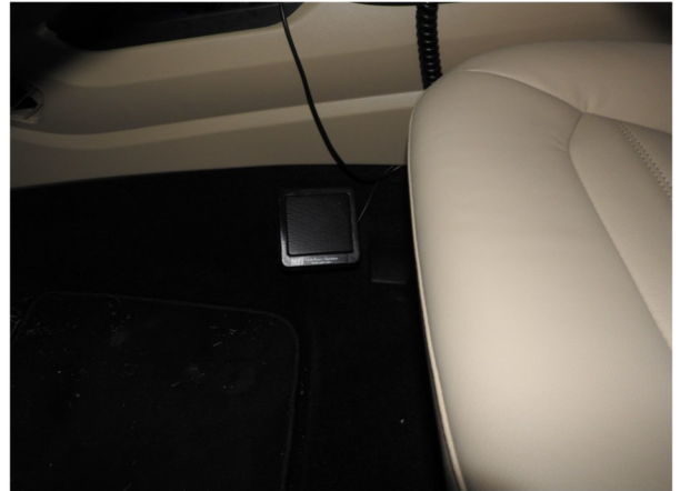
Small external speaker mounted with Velcro to the floor mat below the console and forward of the driver's seat.
