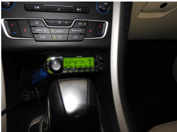
Another view of the control head in place with Industrial Velcro in a 2016 Ford Fusion.
