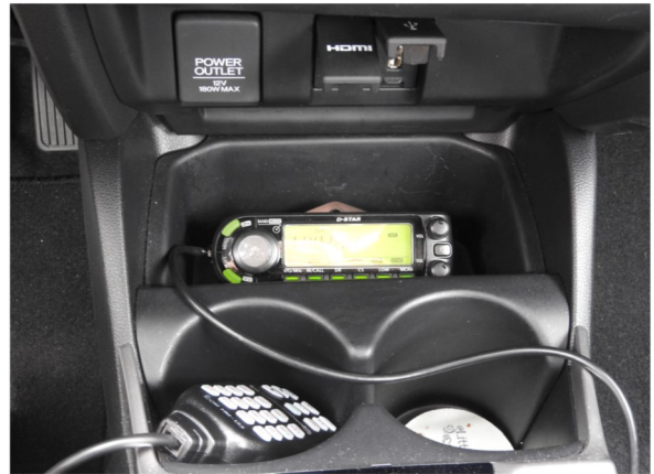
The control head of the Icom 880H mounted with Industrial Strength Velcro under the dash and forward of the center console.
