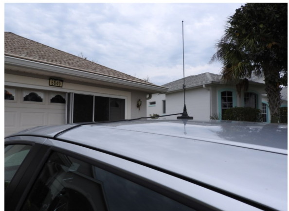
Small quarter wave dual band, magnetic mounted vertical antenna used on both cars.
