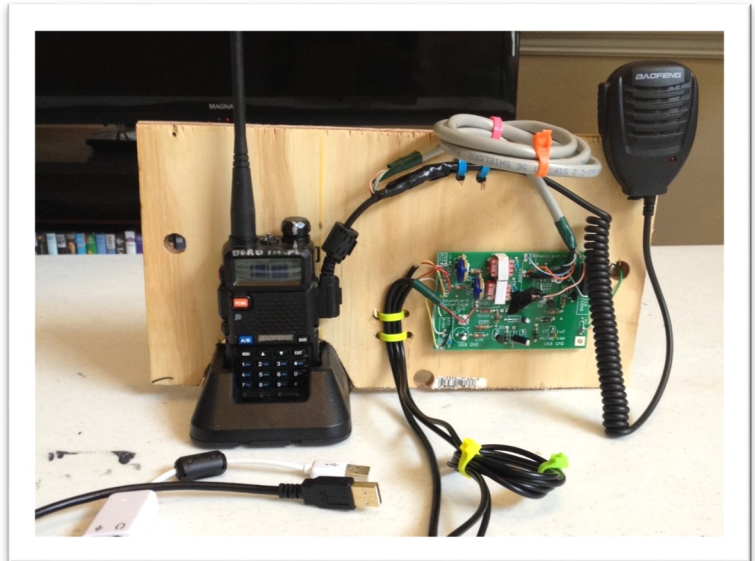
Portable inexpensive voice & digital station useful for training or short-distance emergency communications. Printed circuit board contains simple transistor circuit & transformers to isolate sound card from radio and activate push-to-talk.
