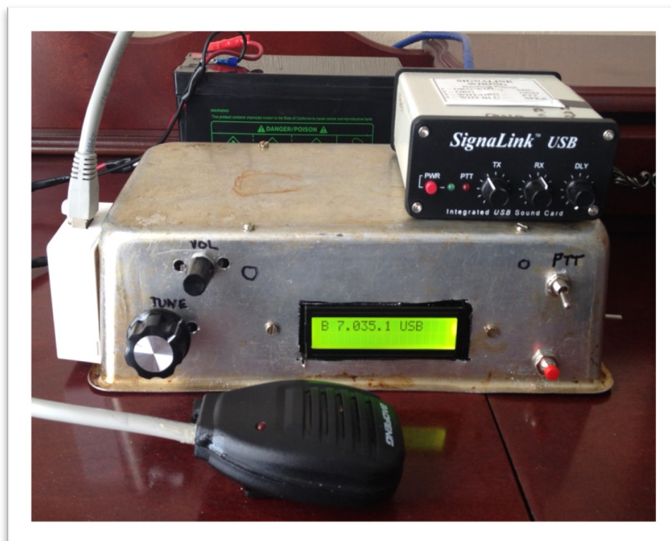
BitX40 enclosed in thrift-shop cake-baking tin; SSB 7-12 watt transceiver can use electret mic or soundcard digital.
