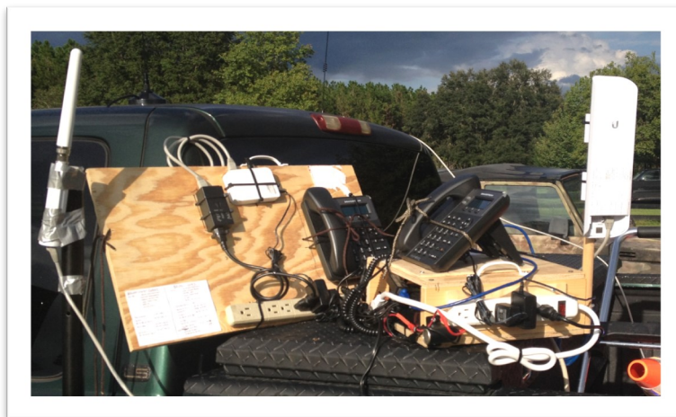
The two microwave systems, one with vertical omni antenna, the more portable unit with pole mounted 10 dB sector antenna. Both systems have network hubs and VOIP telephones.
