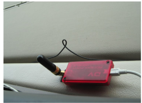
D-Star DVAP placed on the dash of the motorhome and connected to the lap top for contacts using the Icom IC 80 AD hand held.
