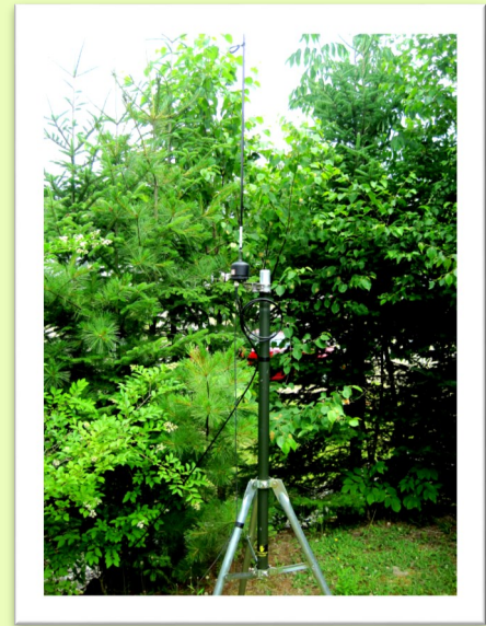
Alpha vertical antenna set up on a TV tripod on a knoll behind the motorhome.
