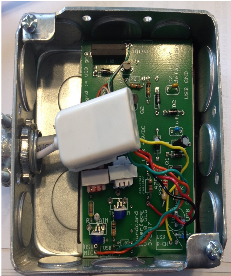
Figure 6. Mounted (actually wedged) into a 2-gang electrical box. One knockout has been removed to allow access to the potentiometers, The USB dongle is also inserted, and another knockout has been removed and a "3/8 non-metallic clamp" used to secure the wires' exit point. There is a standard solid metal plate that fits on top as a cover.
