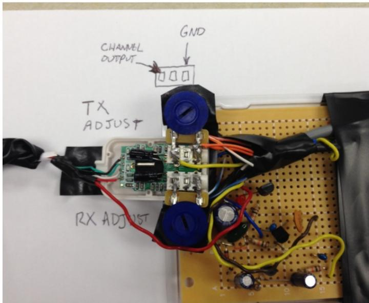
On both the audio output (top) and mic input (bottom), the farthest right terminal is ground, and the farthest left terminal is the signal you want. Solder quickly so you don't melt the entire jack and it will work nicely!
