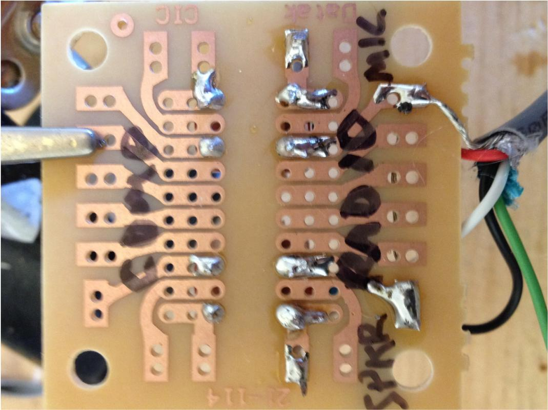
This board layout actually isn't that good for these connections. The 3 pins of the trimmers won't fit because the board isn't drilled on 0.1" centers everywhere. I had to bend the center terminal of the trimmers UP and then I picked these positions for the trimmers to try and make the connections that needed to be made, possible. Be careful not to position the trimmers so that they actually connect to transformer leads that you didn't want them to connect to!
