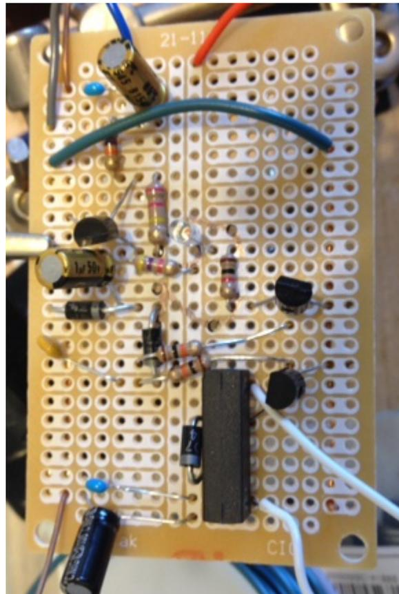
This shows the relay (with pralleled diode) and drive transistor, and the LED indicator circuit. I had to run a short ground wire on this side of the board (that's the jumper green wire going from the other side's ground to this side. You can see the two 10K reisistors coming from the output of the
