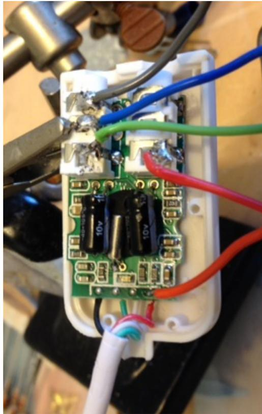
In this photo, the orange wire going near the big white USB cable, is picking off +V from the tiny soldering connection available there. This is a difficult soldering job, be careful. **As an alternative, you can use a second USB cable, just to get to the red and black wires (+v and ground, respectively). This is a lot easier to accomplish mechanically!**
